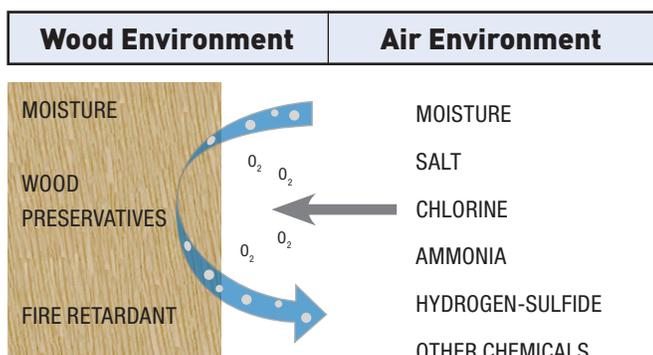
Electrochemical oxidation is the most common type of corrosion affecting metal connectors. It is a process in which iron (Fe) reacts with oxygen (O<sub>2</sub>) in the presence of an electrolyte such as water (H<sub>2</sub>O) to form iron oxide (Fe<sub>2</sub>O<sub>3</sub>), a brown and flaky by-product commonly known as rust.
