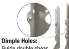
Dimple Holes: Guide double shear nails into the joist and header at a 30° to 45° angle
