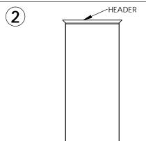
INSTALL HEADER INTO POSITION APPROX. 1" FROM THE TOP AND THE CENTER OF THE ROUGH OPENING.
