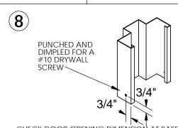
CHECK DOOR OPENING DIMENSION AT BASE OF FRAME (SAME DIMENSION AS BETWEEN JAMBS AT HEADER). SECURE JAMBS WITH DRYWALL SCREW (NOT FURNISHED) THOUGH PUNCHED AND DIMPLED HOLE AT THE BASE OF FRAME. BE SURE TO ATTACH SCREWS TO BOTH SIDES OF BOTH JAMB LEGS (4 PLACES).
