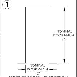
ADD TO DOOR OPENING DIMENSIONS: 2" TO WIDTH AND 1" TO HEIGHT. FOR A 3070 DOOR FRAME, THE ROUGH OPENING IS 38 "  $\times$  85".
