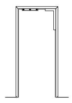
IF FEASIBLE, HANG DOOR NOW AND ADJUST FRAME ON WALL TO ALLOW PROPER DOOR / FRAME CLEARANCES OR PLUMB FRAME WITH CARPENTER SQUARE AND/OR LEVEL. (ADJUST HEADER LEVELNESS BY SHIMMING UNDER JAMBS).
