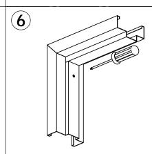
TURN ADJUSTING SCREWS IN BOTH JAMBS COUNTERCLOCKWISE UNTIL ANCHOR IS RESTING AGAINST THE WALL.
