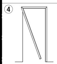
REPEAT STEP #3 WITH HINGE JAMB. PULL HEADER DOWN TIGHTLY ONTO JAMBS. LOCK HEADER AND JAMBS TOGETHER BY BENDING OVER EXPOSED TABS.
